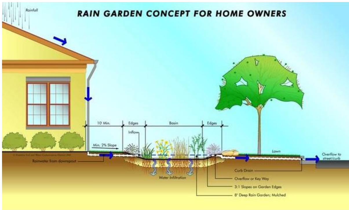
Figure 3.12: Configuration of a rain garden
