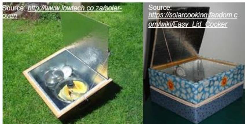
Figure 3.33: Box type solar cooker (left), and Easy Lid cooker (right)
